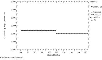
**Figure 1.7.2.2** CTD #4 conductivity slope corrections by station number.
