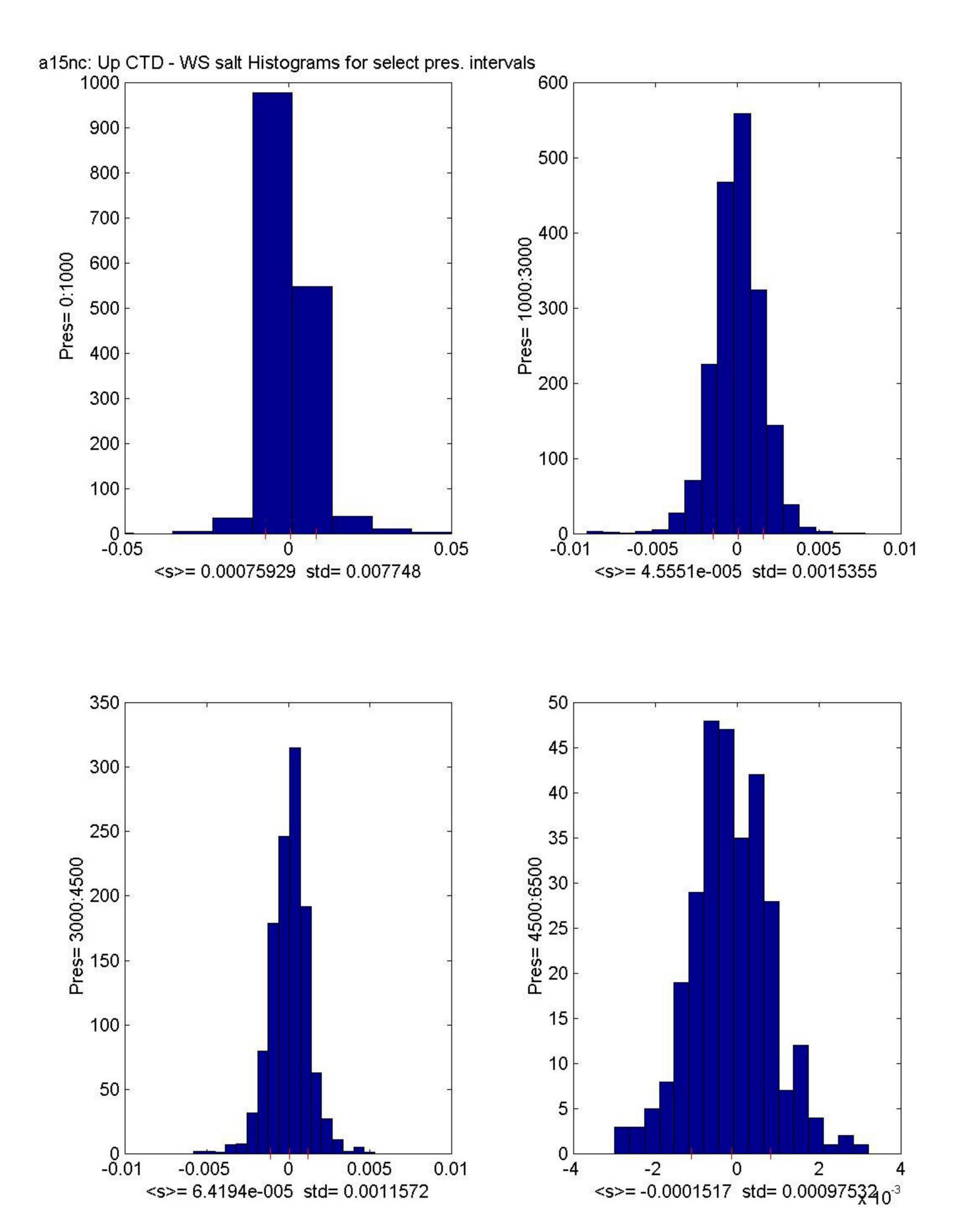
Figure 10: 4 histogram panels of up cast salinity differences Ds = (CTD-WS) psu for various pressure intervals as labeled.
