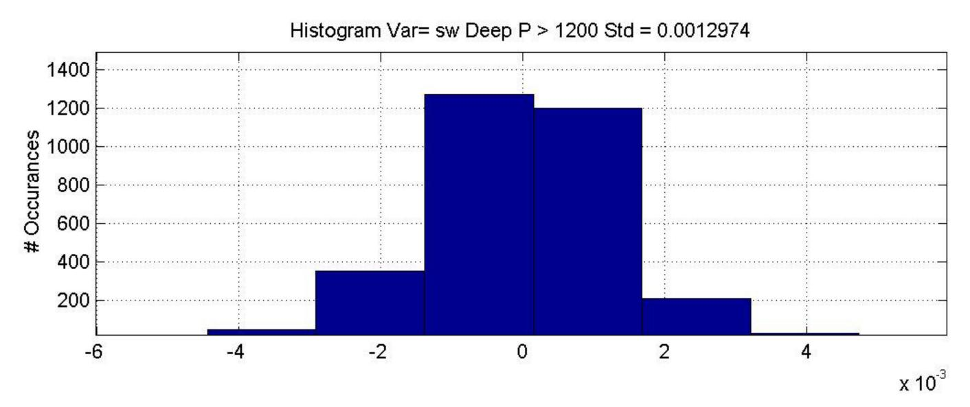
Figure 6: Histograms of QUAL1 "good" water sample salinity differences (CTD-WS) psu.
