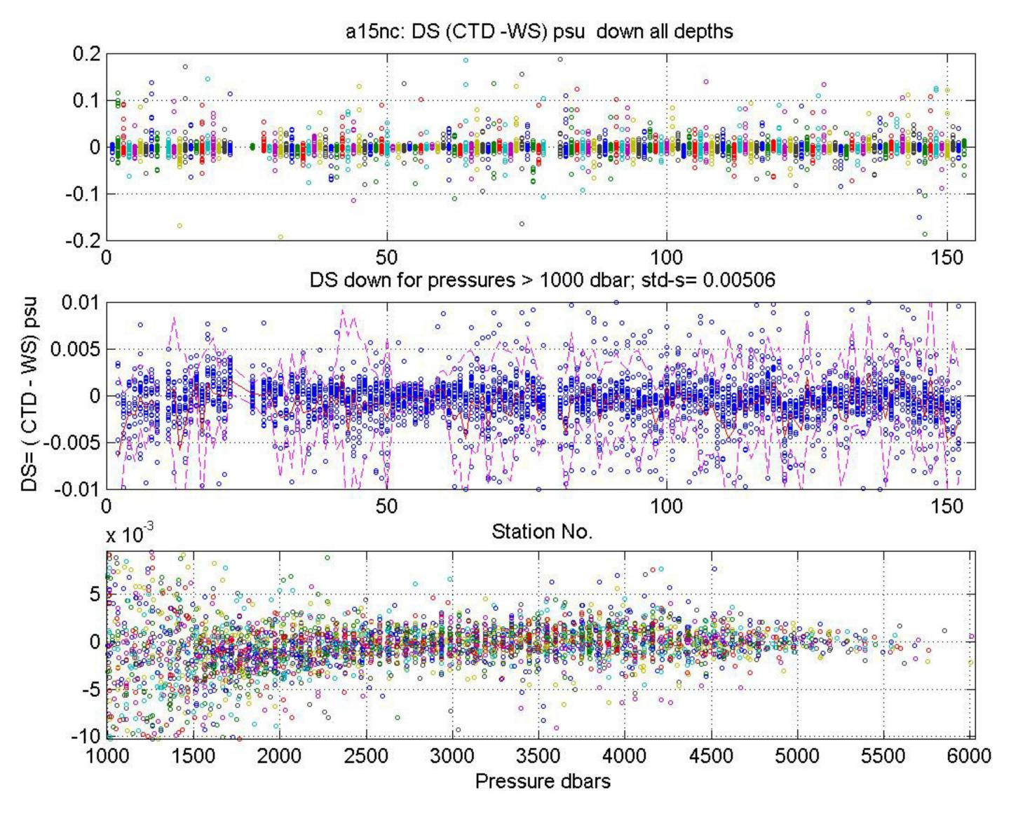
Figure 9: 3 Plot panels of downcast salinity differences Ds = (CTD-WS) psu versus station number
