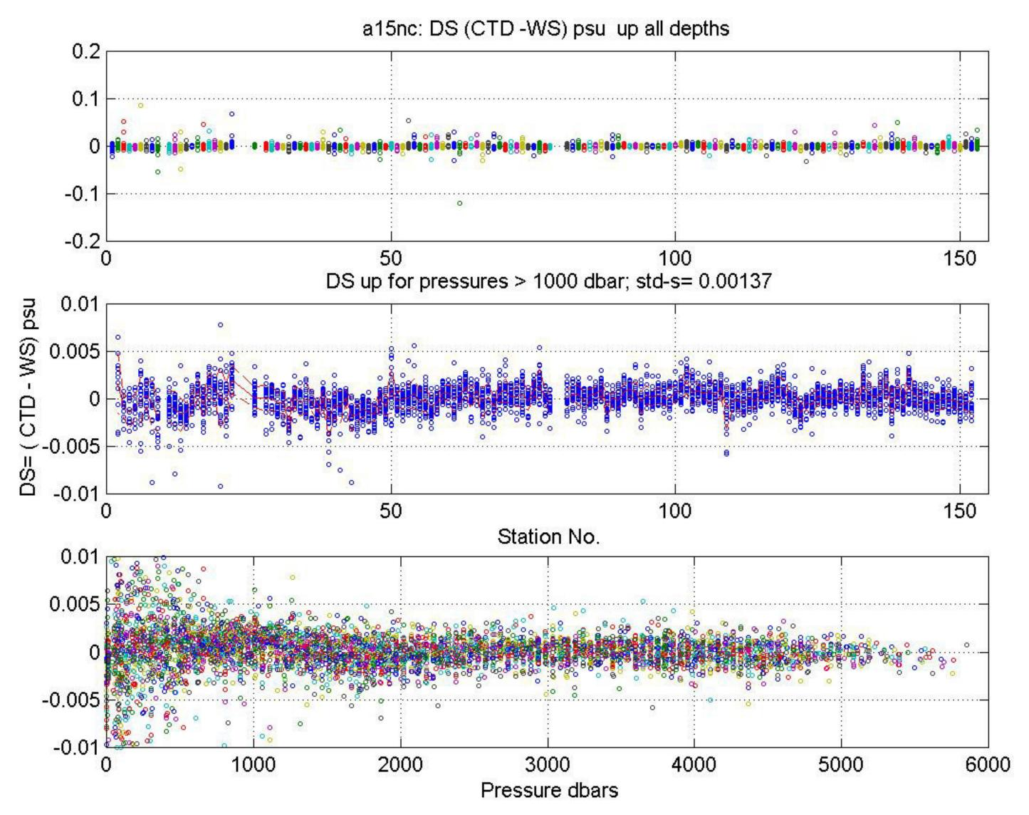
Figure 8: 3 Plot panels of up cast salinity differences Ds = (CTD-WS) psu versus station number
