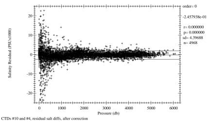
Figure 1.7.2.4 Salinity residual differences vs pressure (after correction).
