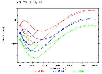
Figure 1.6.1 Pressure calibration for ODF CTD #10, July 1994.
