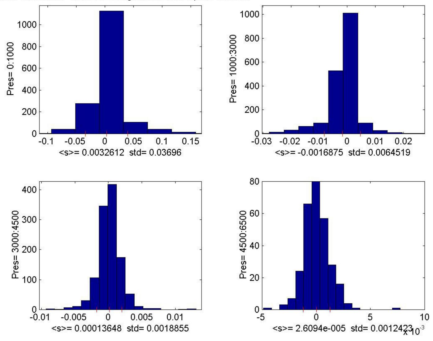
Figure 11: 4 histogram panels of downcast salinity differences Ds = (CTD-WS) psu for various pressure intervals as labeled. Note a much higher standard deviation in 2 shallowest histogram panels compared to up cast.
