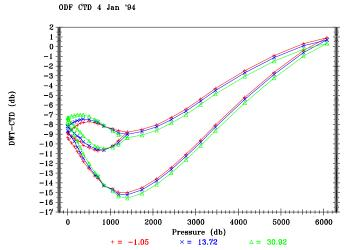
Figure 1.6.2 Pressure calibration for ODF CTD #4, January 1994.
