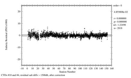
**Figure 1.7.2.6** Deep salinity residual differences vs station # (after correction).
