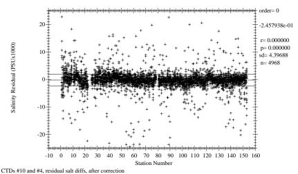
Figure 1.7.2.5 Salinity residual differences vs station # (after correction).
