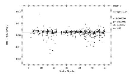
Figure 1.7.1.0 Shipboard comparison of CTD #10 primary/secondary PRT channels, pressure>1000db.
