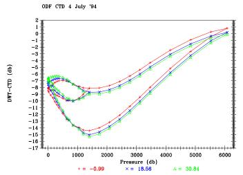
Figure 1.6.3 Pressure calibration for ODF CTD #4, July 1994.
