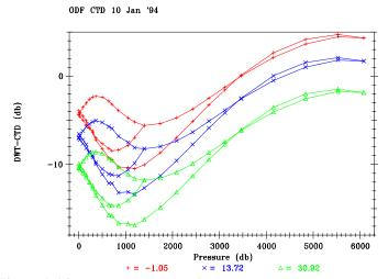
Figure 1.6.0 Pressure calibration for ODF CTD #10, January 1994.
