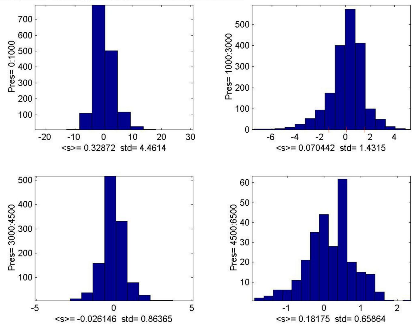
Figure 13: 4 histogram panels of up cast oxygen differences Dox = (CTD-WS) in µmol/kg for various pressure intervals as labeled.
