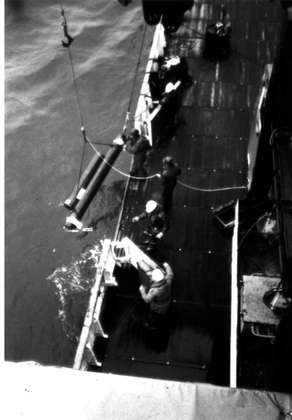
Fig. 5: Deployment of RAFOS sound source (IfM Nr. V385) on Station 231.
