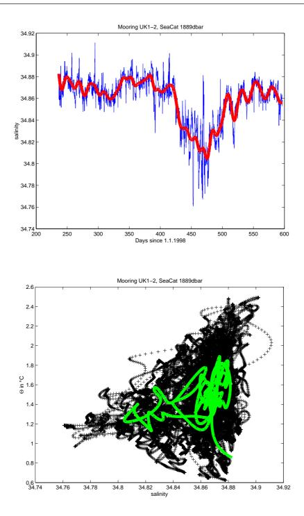
**Fig. 60:** Data from the SeaCat instrument located in the Denmark Strait Overflow Water at section 3. a) Salinity as a function of time (the thick line is is low-pass filtered data) b)  $\theta$ /S diagram (the line being the low-pass filtered data).
