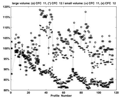
Figure 2: Temporal evolution of the ECD-effciency during the cruise for the 0.5 mL volume (small) and the 2 mL volume (large).
